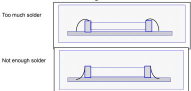
Cracks tend to occur due to large stress.
